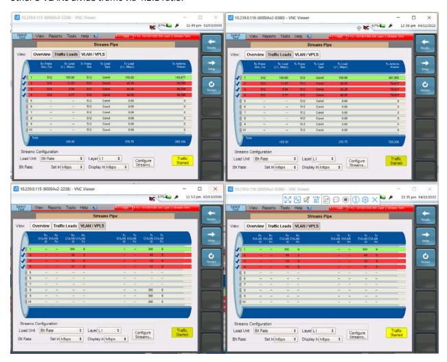
It looks like the QOS is working even though the P-bits are not all correctly being shown at the receiving tester.
